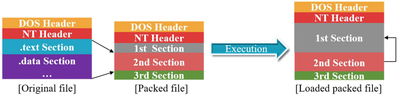
Fig. 1. Overview of packing the original program and executing the malware.
