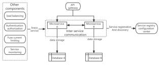
Fig. 2. Microservice architecture.
