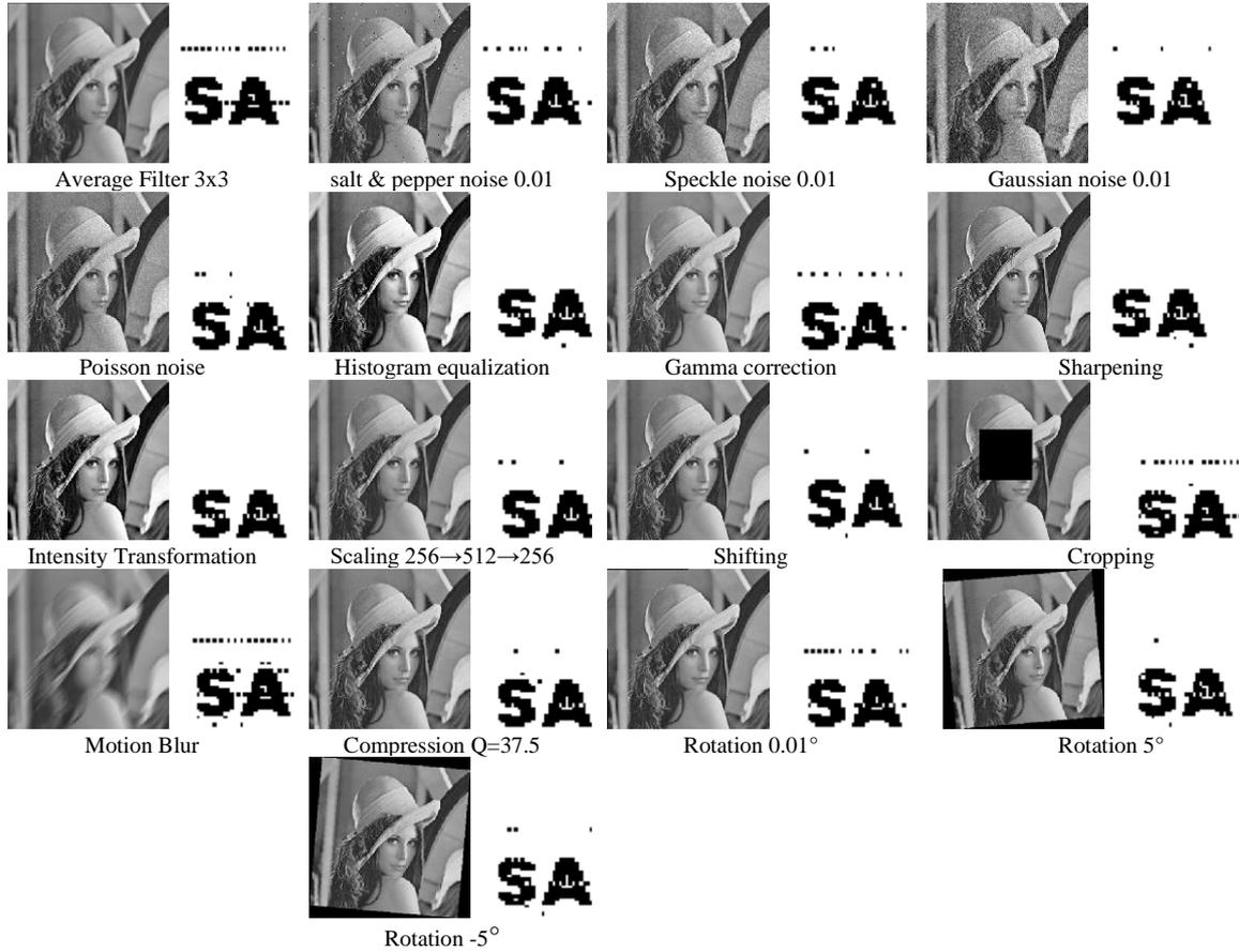
Fig. 3. Attacked watermarked images and extracted watermarks.
