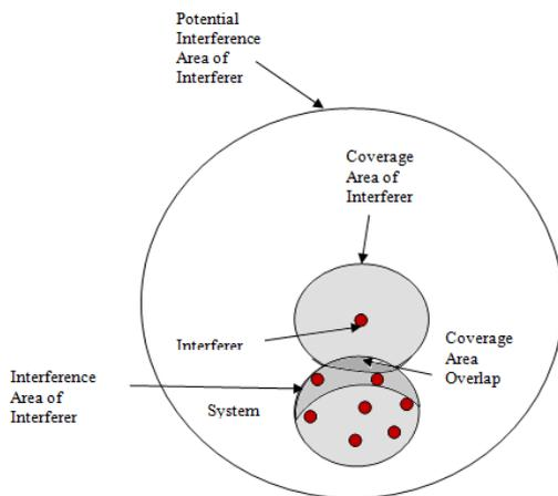
Fig. 1. Coexistence system geometrical model.
