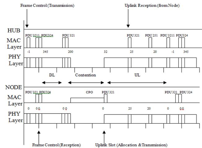
Fig. 2. The frame format of IEEE 802.16 standard.
