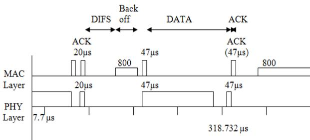
Fig. 3. Data Exchange of IEEE 802.11 Standard.
