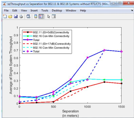
(a) Throughput vs Separation for 802.11 & 802.16 Systems without RTS/CTS (Minimum connectivity)
