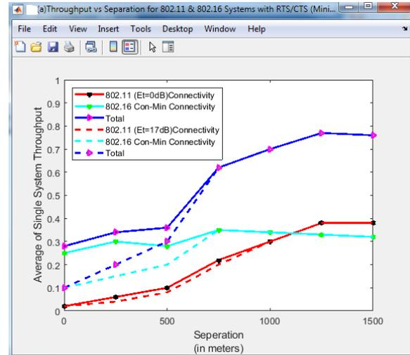
(a) Throughput vs Separation for 802.11 & 802.16 Systems with RTS/CTS (Minimum connectivity)
