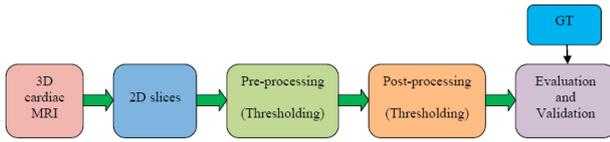
Fig 1. Various stages existing in the proposed Computerized Image Examination System.
