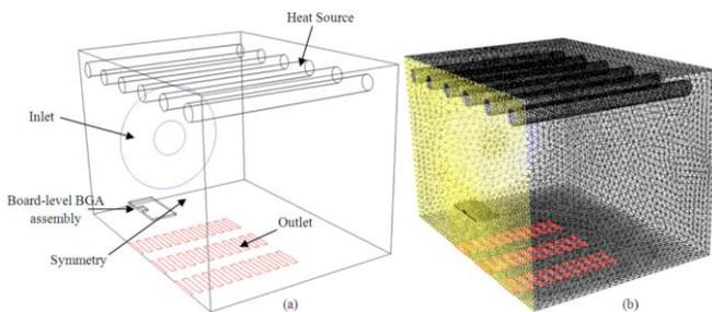
Fig. 1. (a) Three-dimensional half geometry of the reflow oven without the board-level BGA assembly. (b) Meshed with hexahedral grid
