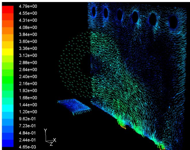
Fig. 6. Velocity vector around the reflow oven at 200s (Unit: m/s)
