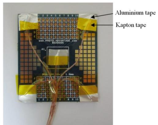
Fig. 4. Location of the thermocouple attachment on the PCB
