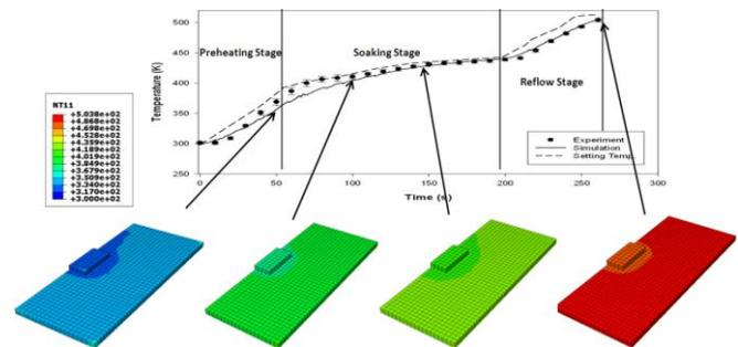
Fig. 8. Temperature distribution contour of the half board-level BGA assembly (Unit: K)
