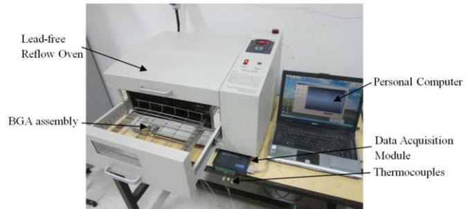
Fig. 3. Experiment setup
