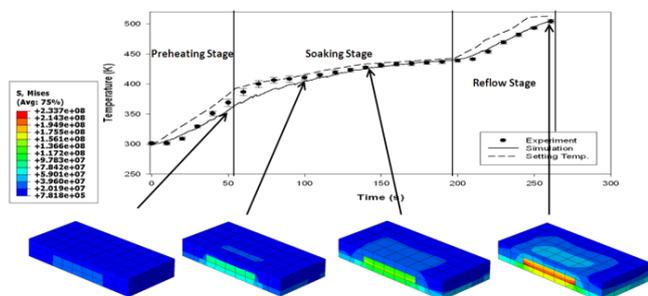
Fig. 9. Von-mises stress contour on BGA assembly (Unit: Pa)
