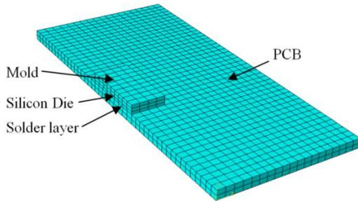
Fig. 2. Computational meshes in the board-level structural model
