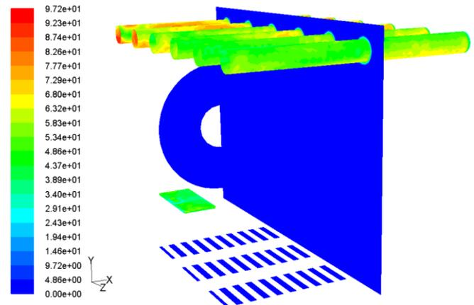
Fig. 7. Surface heat transfer coefficient contour of half of reflow oven. (Unit: W/m<sup>2</sup>.K)
