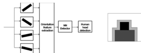
Fig. 4. Neuromorphic vision for human detection, inspired by the visual cortex, and based on the neural network detector of head-torso shape.
