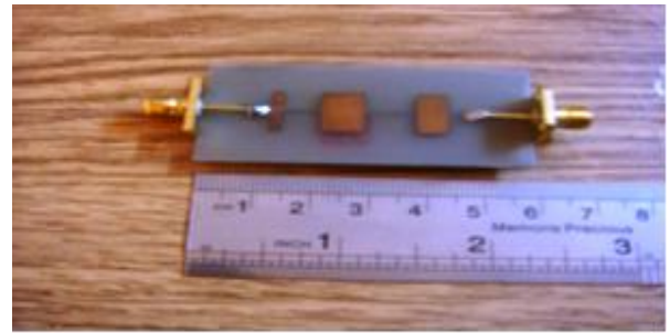
Fig. 6. Photo of micro strip filter built on the substrate with a dielectric constant 4.2 and thickness 1.58 mm.
