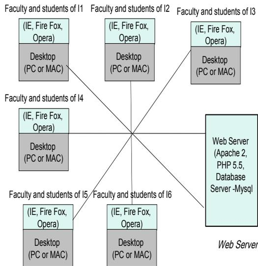
Fig. 1. Server based architecture
