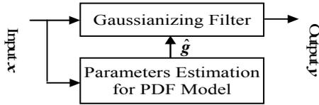
Figure 1. Block diagram of gaussianizing filter
