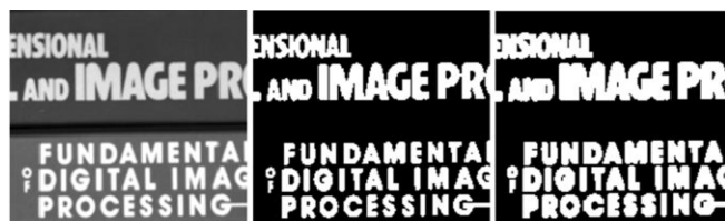
Fig. 3. (a) Gray Scale image, (b) Binary Image by thresholding, (c) Dilation: a 2x2 square structured [4].
