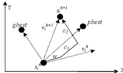
Fig. 3. The velocity and position updates in PSO.
