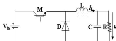
Fig. 1. Buck DC-DC converter.
