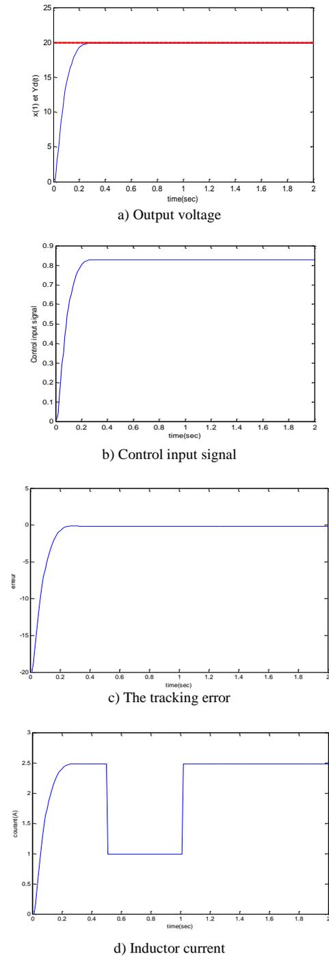
Fig. 5. Simulation results for converter with load fluctuation.
