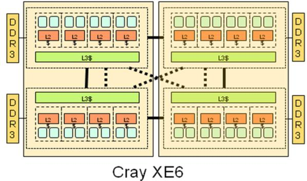
Fig. 1. NUMA architecture at Cray XE6 nodes.
