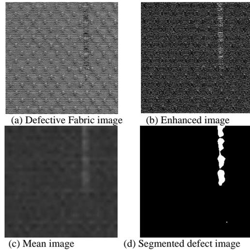
Fig. 2. The steps of defects segmentation algorithm
