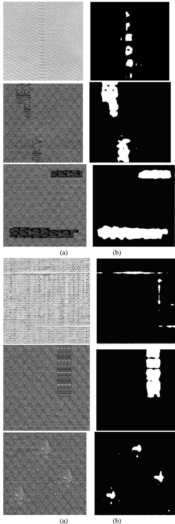
Fig. 4. Segmentation result of some patterned and unpatterned defects image, (a) defect image; (b) segmented image
