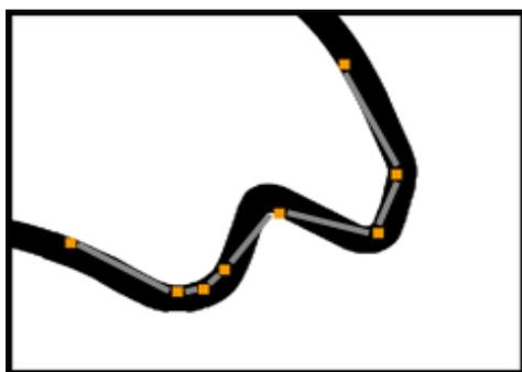
Fig. 9. More waypoints needed in sharp curve.
