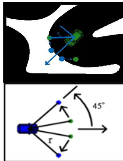
Fig. 7. New collision detection points when Figure 6's two collision detection points are activated at the same time.
