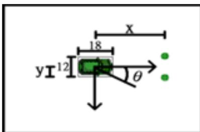
Fig. 6. Collision detection points of car.
