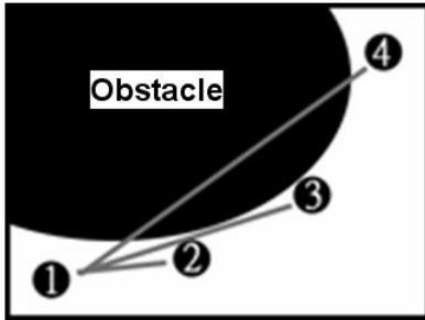
Fig. 4. Modified A\* algorithm by a line-of-sight algorithm.
