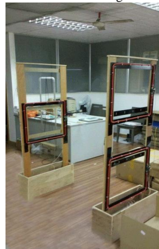
(a) The antenna construction in wood structure
