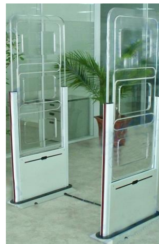
(b) The antenna prototype in organic glass.
