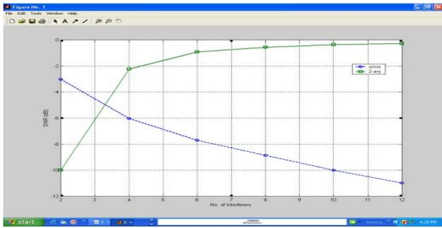
Fig. 6. SINR vs. No. of interferers for omni-directional antenna and 2-element adaptive antenna array
