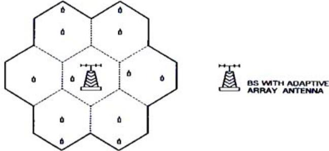
Fig. 2. Proposed WCDMA mobile environmental deploying adaptive array antenna at BS
