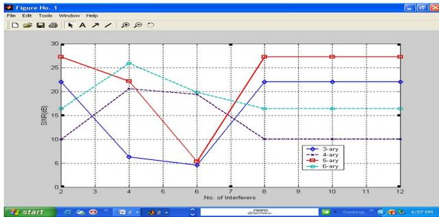
Fig. 7 (a) . comparative analysis of SINR for lower-element array
