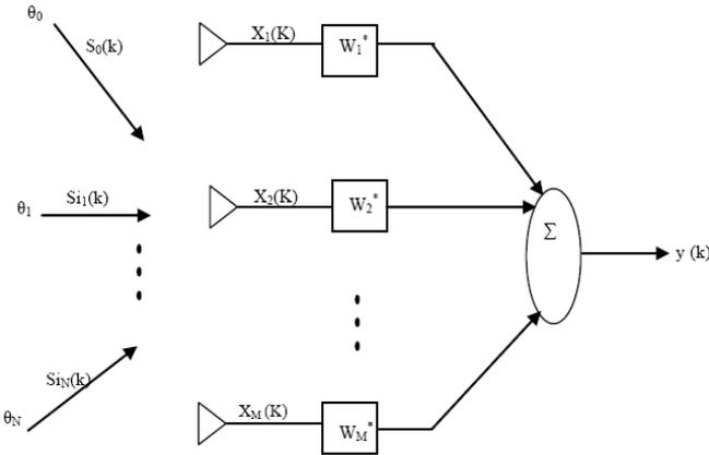
Fig. 3. Conventional narrowband beam forming array
