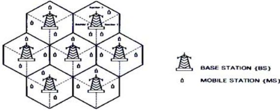
Fig. 1. Typical WCDMA mobile environment with sector antenna at BS
