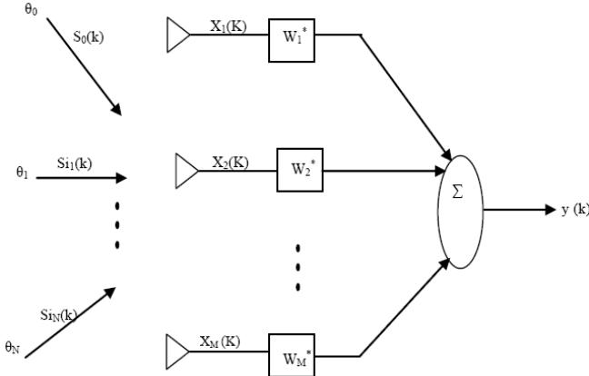
Fig. 3. Conventional narrowband beam forming array
