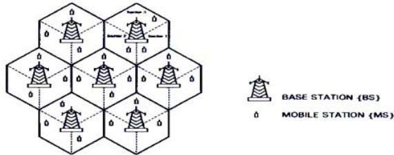
Fig. 1. Typical WCDMA mobile environment with sector antenna at BS
