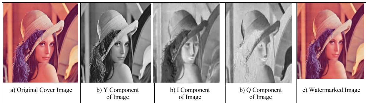
Fig. 4. Original color lena image with 5212 × 512 size, Y, I, Q components and watermarked image.
