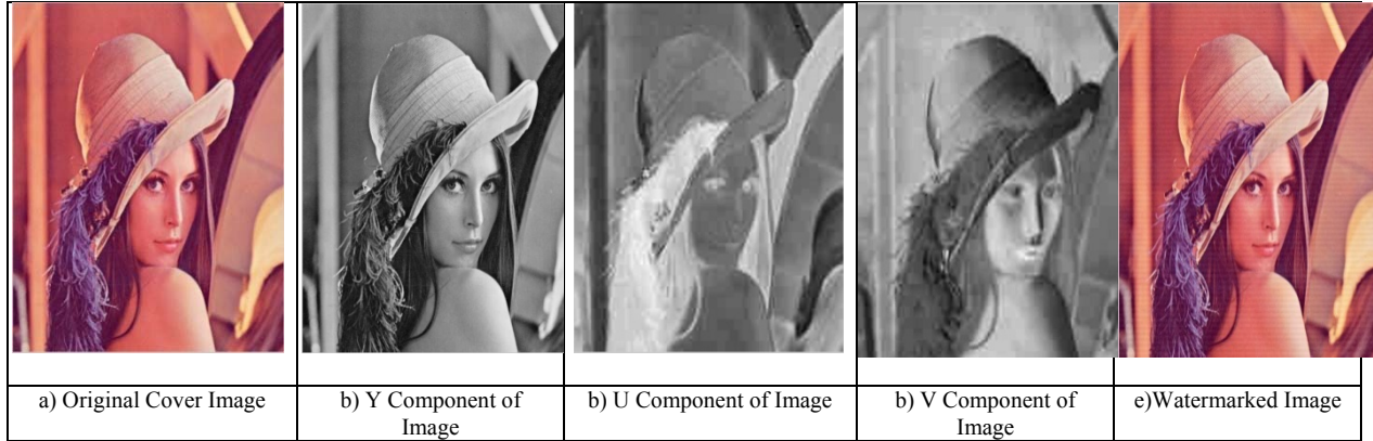
Fig. 2. Original color lena image with 5212 × 512 size, Y,U,V components and watermarked image.
