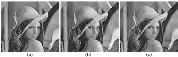
Fig.10. ROI encoding in real world image (a) original Lena image with uniform resolution (b) Compressed image (0.2 bpp) (c) Encoded image using proposed ROI encoding (1 bpp for ROI and 0.2 bpp for background)
