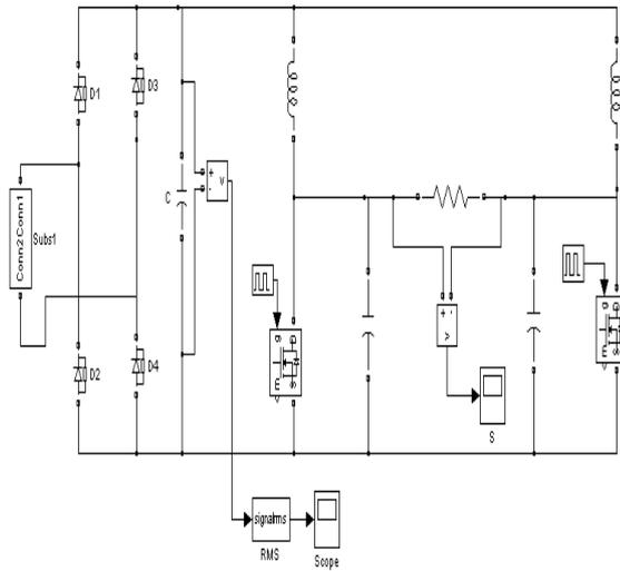
Fig.4a. Matlab Simulation circuit
