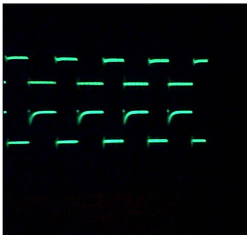
Fig. 5b Driving pulses for S1 & S2
