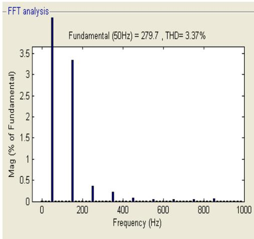
Fig 4.g FFT Analysis for output voltage
