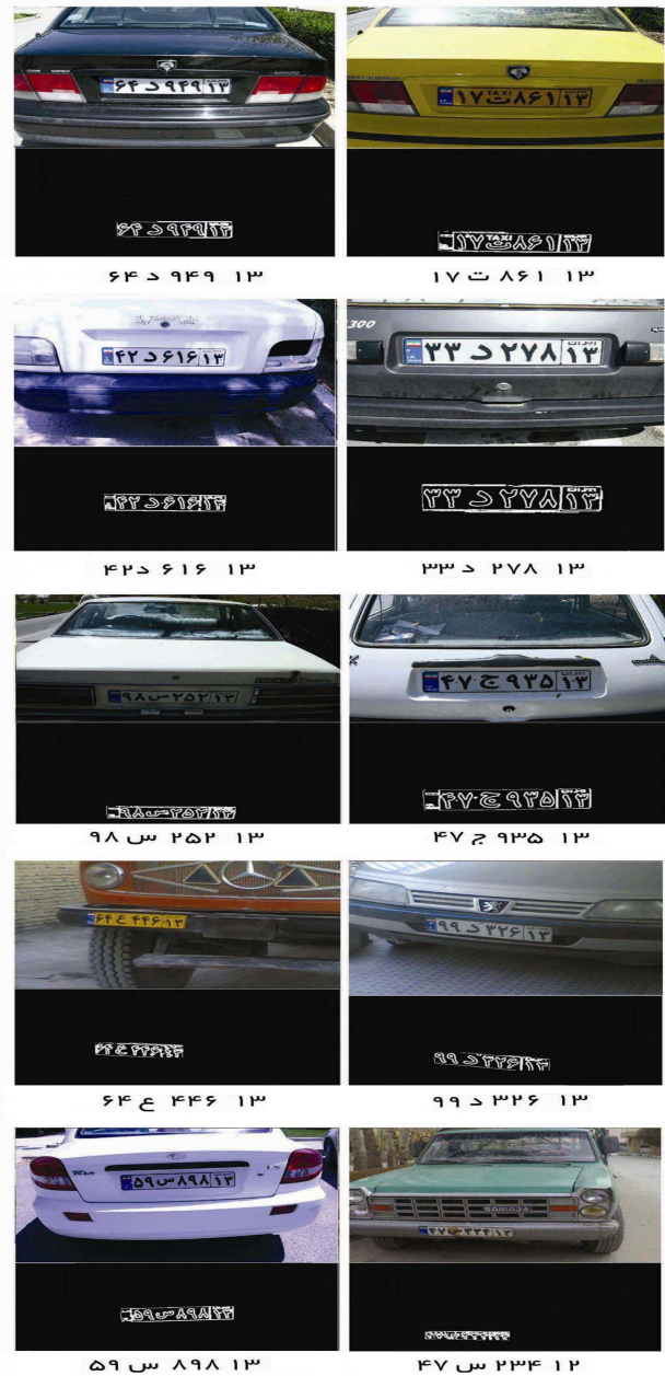
Fig 6. The outcomes of the LPR system, car images, localized car plate, and recognized characters in different test images
