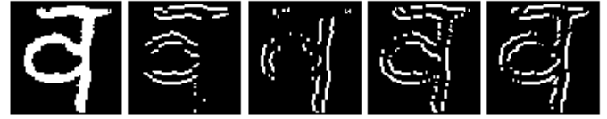
Fig. 5 Four sub-images (right side) obtained using four Kirsch operators (4-7) and fifth sub-image (left side) obtained due to original image, Fig. 4(a), after normalizing its size to 70 \times 70 pixels.
